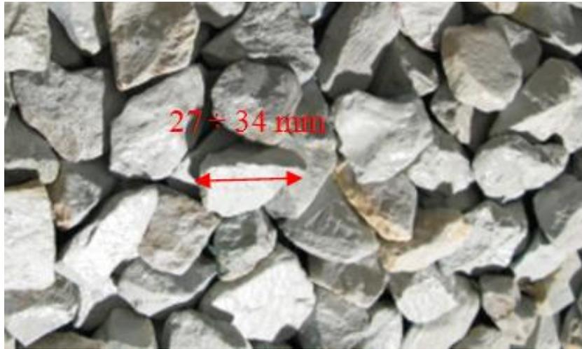
Figure 61: Rocks used for armour layer.
