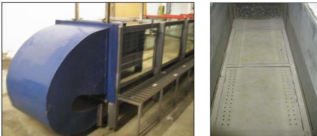
Figure 49: Left: Diffuser at the bottom of the flume. Right: The bottom of the channel.
