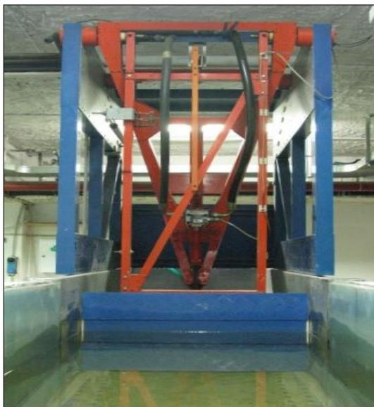
Figure 50: Front perspective of the mechanical part of the wave maker.
