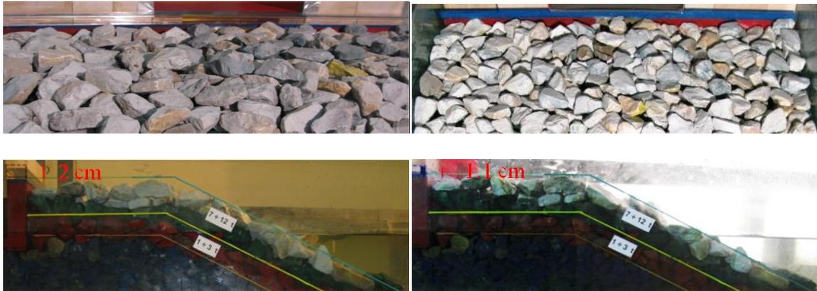
Figure 65: Raising the wave wall in configurations C4 and C5.
