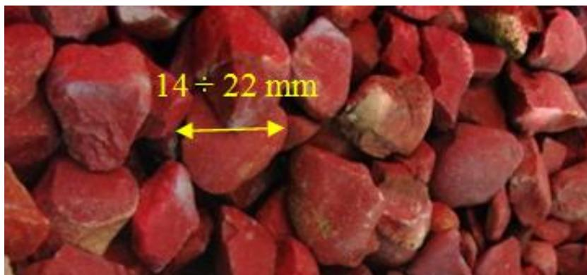
Figure 62: Rocks used for filter layer.
