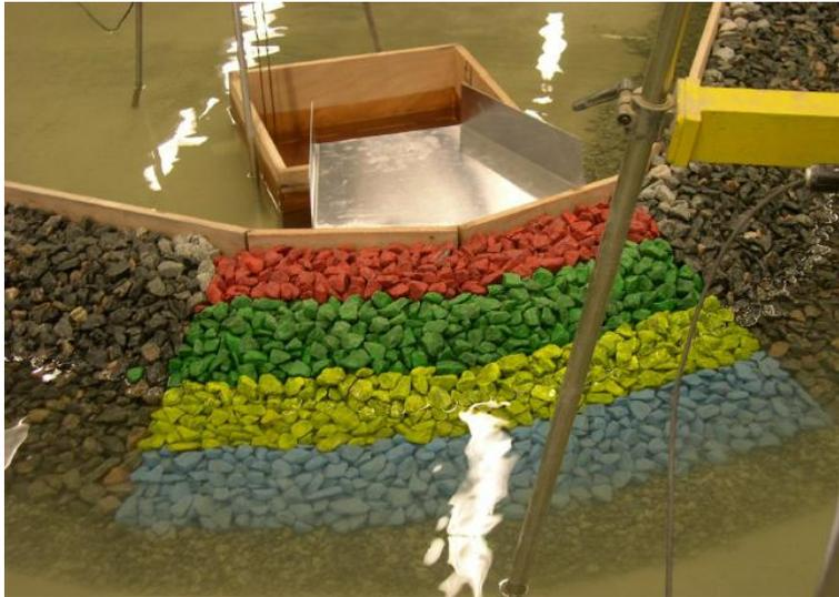
Figure 45: Measurement of wave overtopping using an overtopping tank.
