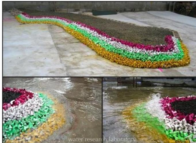
Figure 43: Typical three-dimensional coastal structure model in wave basin.
