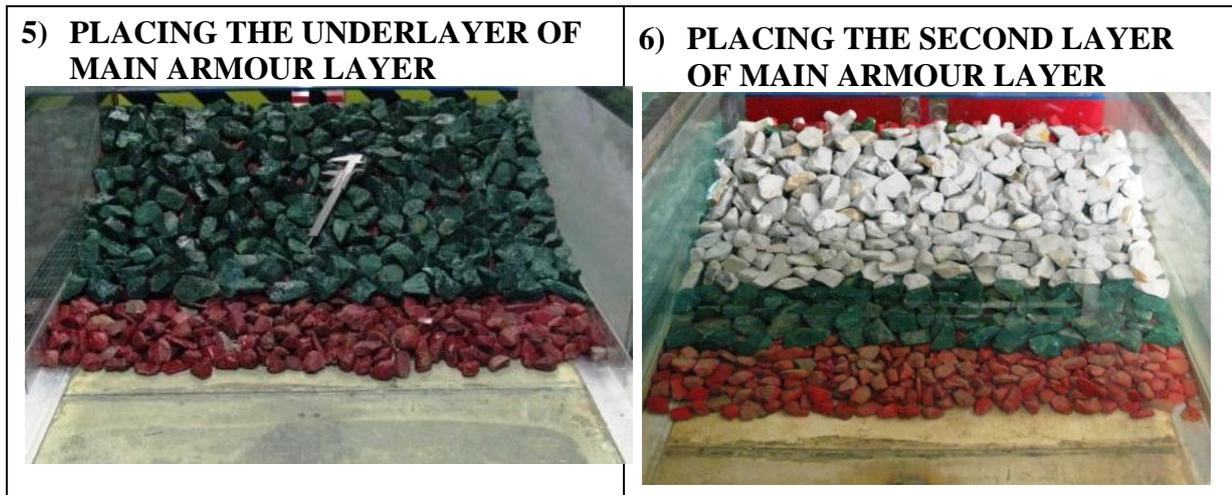
Figure 68: Construction phases of the harbour breakwater in the wave flume.
