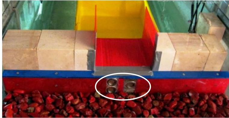
Figure 46: Pressure sensors installed inside the wave wall.
