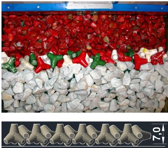
Figure 64: Placing tetrapods into the model.
