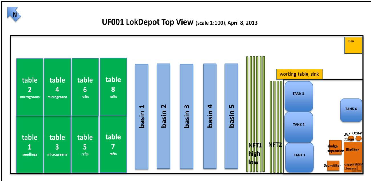
Figure 5: Floor plan of the world's first commercial rooftop aquaponic farm: UF001 LokDepot in Basel.
