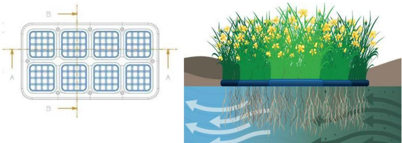
Figure 2: Tech-IA floating element and its working scheme
