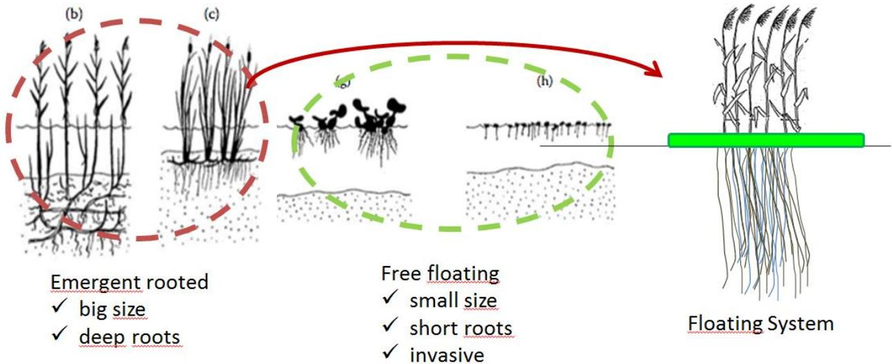
Figure 1: The concept of the floating system
