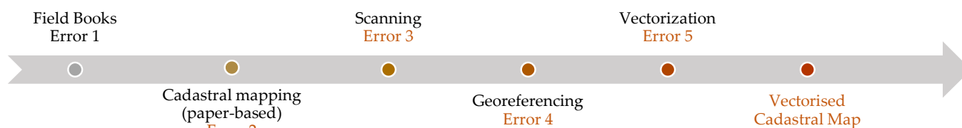
Figure 4. Digitisation of analogue cadastral maps in North Macedonia and Slovenia. Field books with measurement data were not considered in this process.
