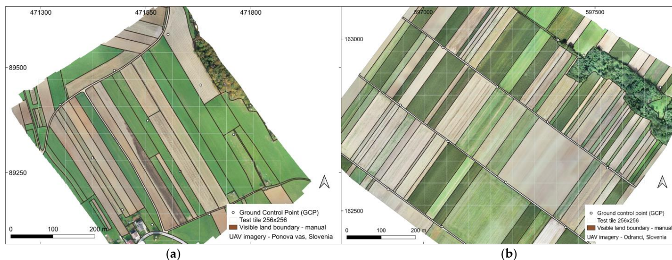
Figure 3. Manually delineated visible land boundaries; (a) UAV orthoimage with ground sampling distance (GSD) of 0.25 m Ponova vas, Slovenia; (b) UAV orthoimage with GSD of 0.25 m for Odranci, Slovenia; (a,b) (EPSG 3794).
