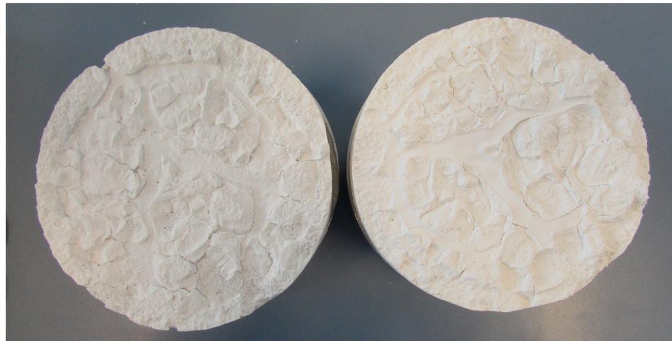
**Figure 8.** Disc-sandwich model after the adhesion test; grout LS injected into 5 mm air pocket.
