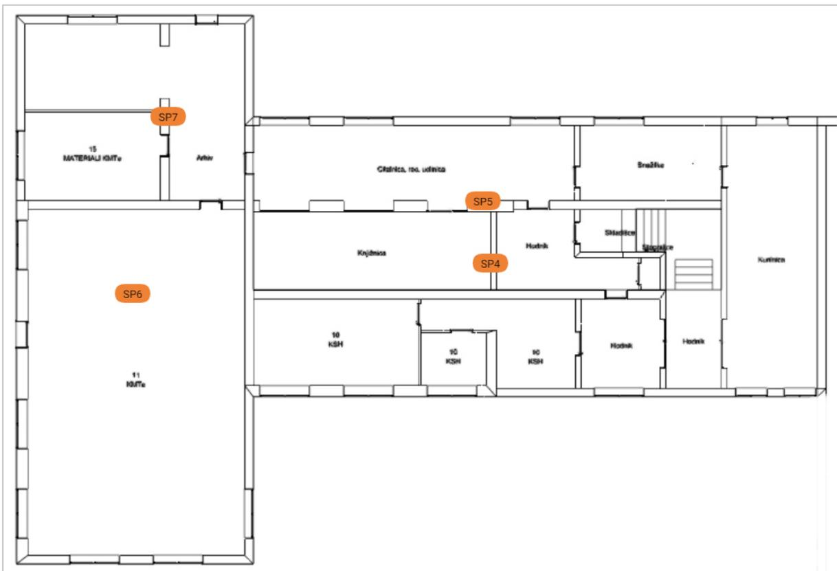
Figure 34. Placement of IAQ Sensors in the Basement
