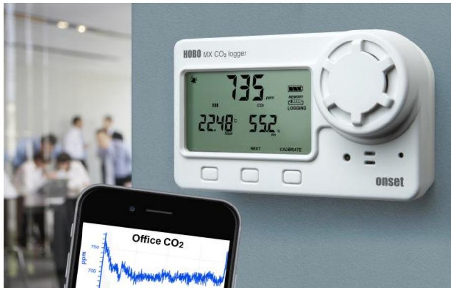
Figure 14. Data logger MX1102A (HOBO Onset, 2019)
