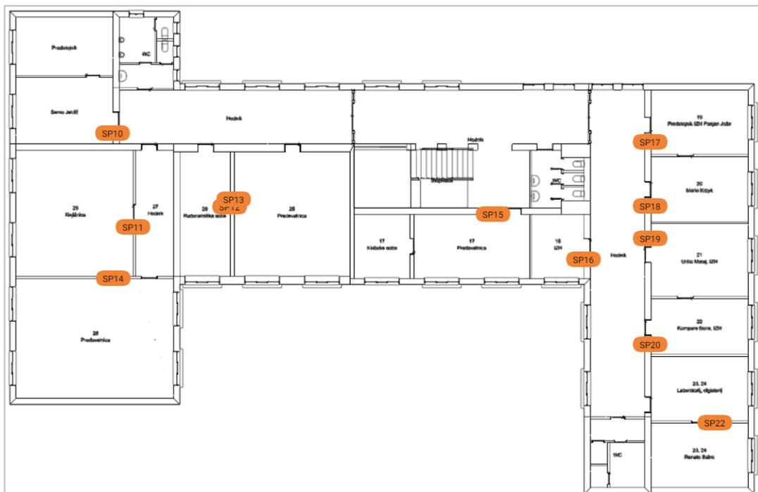
Figure 36. Placement of IAQ Sensors in the First Floor
