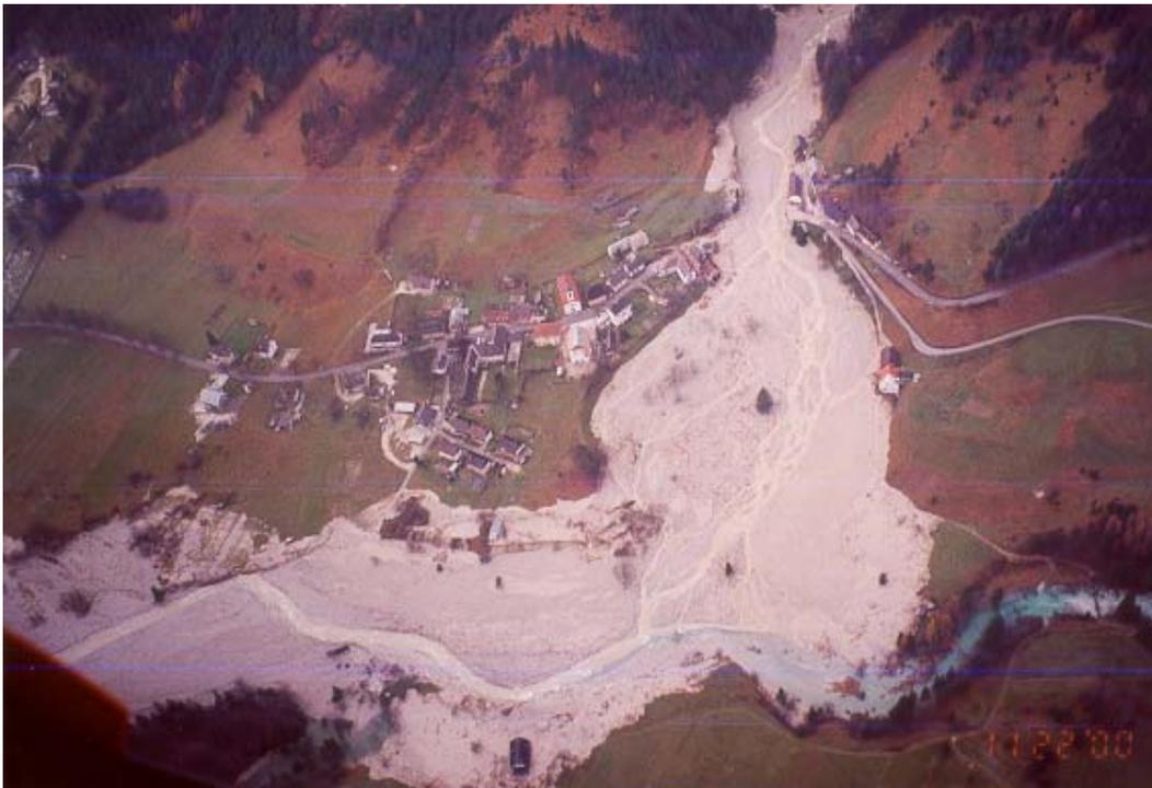
Figure 6. Helicopter view of the debris flow deposits in Log pod Mangartom after the devastating debris flow in November 2000 – the Predelica Torrent flows from above into the Koritnica River, coming from the right.
