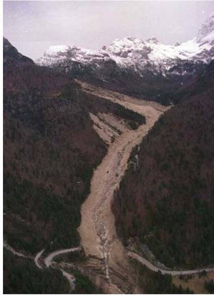
Figure 5. Helicopter view of the debris-flow pathway from the source area on the Stože slope across the regional road Bovec-Tarvisio (Italy).
