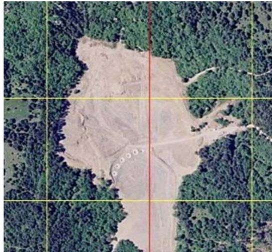
Figure 16. The upper part of the Slano Blato landslide with partially finished reinforced concrete deep wells on its right-hand side (square is 100 x 100 m).
