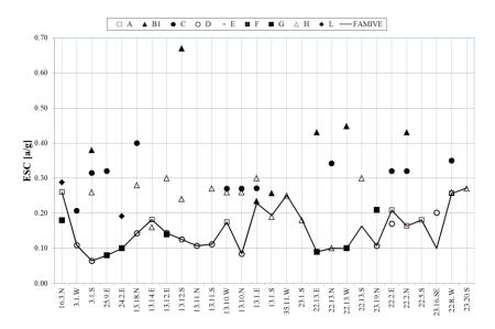
**Figure 4.** Evaluated Equivalent Shear Capacity (ESC) for 33 case studies and comparison between observed and calculated critical mechanisms
