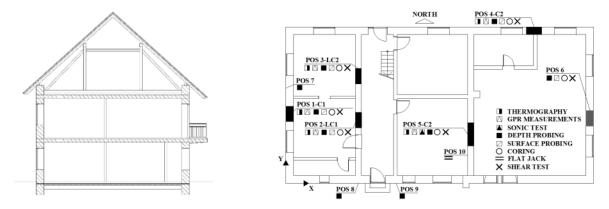
Figure 9. Cross-section of typical stone masonry building and in-situ testing positions
