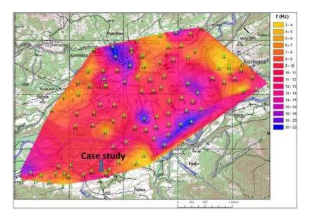
**Figure 13.** Map for Bovec basin of the fundamental frequency peaks derived through microtremor measurements (Gosar, 2007)
