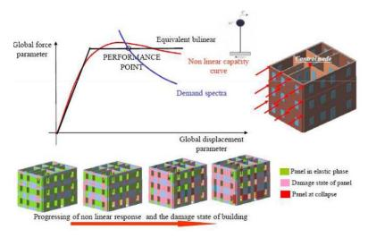
**Figure 2.** Identifying performance point through GMR considering seismic demand (Lagomarsino et al., 2011)
