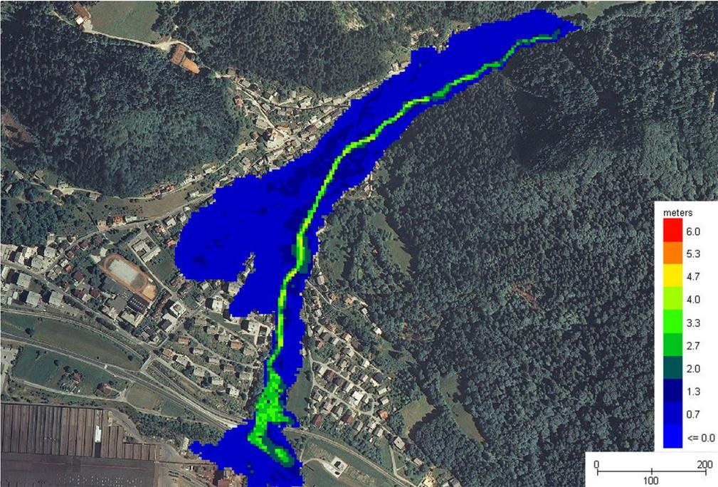
**Fig. 7** Maximum flow depths using DEM5 (re-sampled LiDAR data)
