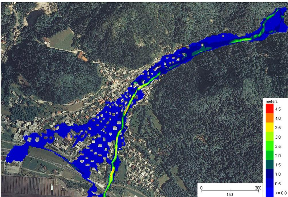
**Fig. 2** Maximum depths using blocked (“dry”) cells for representing structures.
