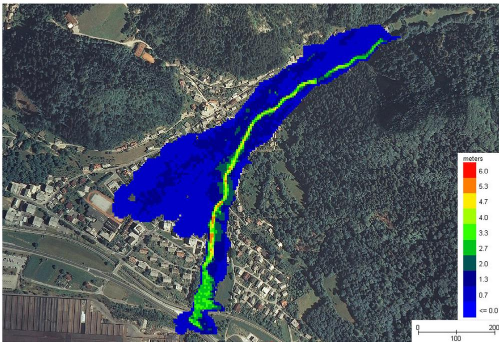
**Fig. 6** Maximum flow depths using DEM0.5 (original LiDAR data)
