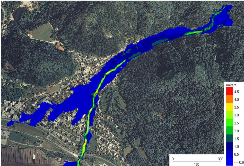
**Fig. 1** Maximum depths using higher Manning coefficient for representing structures.
