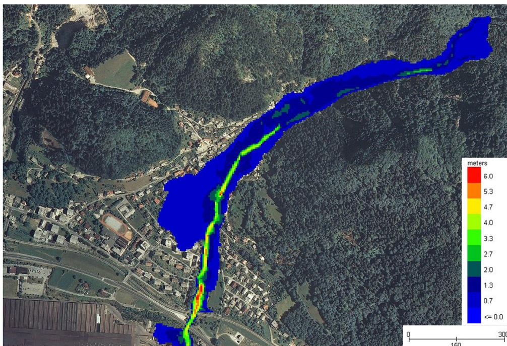
**Fig. 4** Maximum flow depths using classical DEM5
