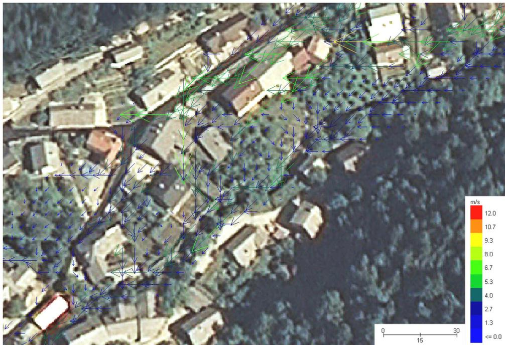
**Fig. 3** Maximum velocities (vectors) using blocked (“dry”) cells for representing structures (the upper part of the fan).
