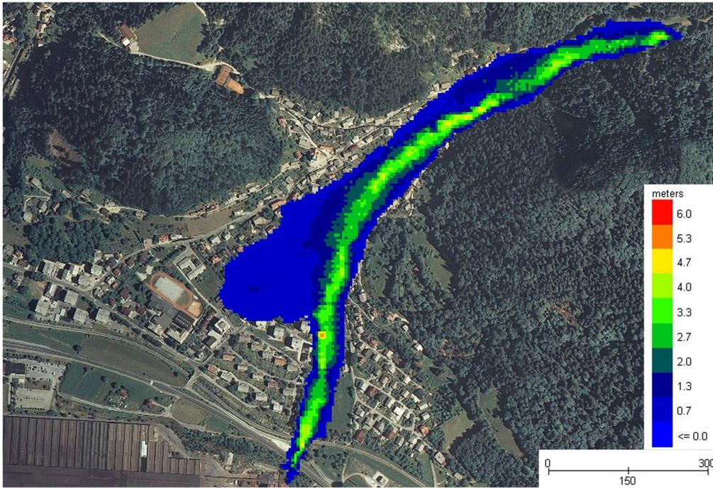
**Fig. 5** Maximum flow depths using classical DEM12.5
