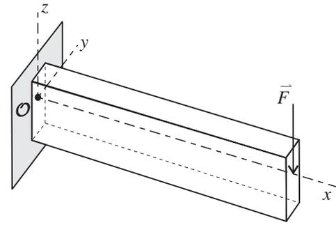
**Figure 5** : Lateral buckling of a cantilever.
