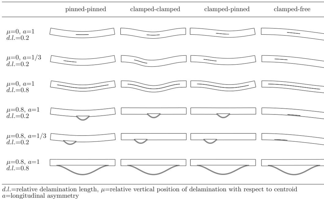
Fig. 5. Buckling modes of various delaminated columns.
