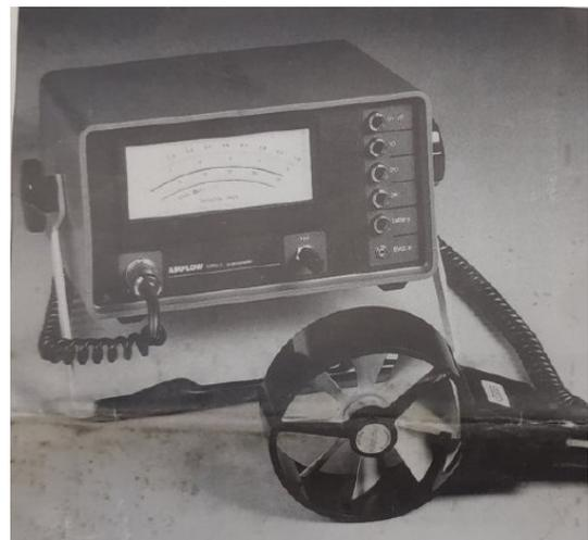
Figure 5.20: Vane anemometer.
