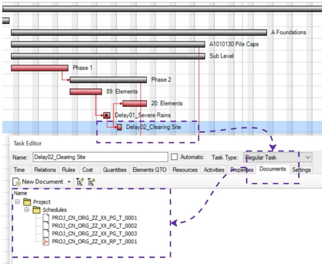
Figure 48: Attaching documents to the delay activity within the Task Editor
