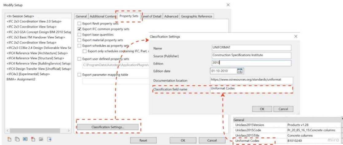
Figure 21: Input of Classification Codes in Revit and linking it for IFC Export
