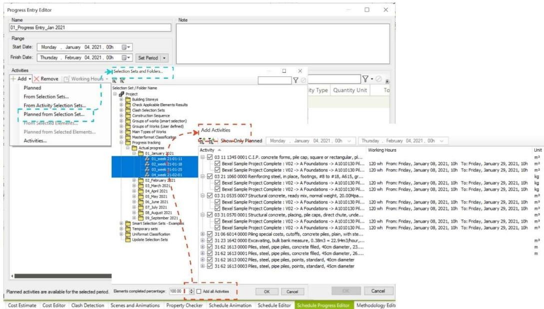
Figure 42: Method of Progress Entry in Bexel Manager
