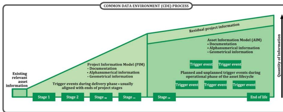
Figure 15: Data gathered during a project lifecycle according to ISO 19650-1
