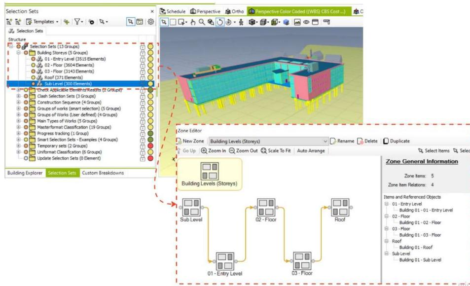
Figure 31: Selection set based on the levels or storey in the building
