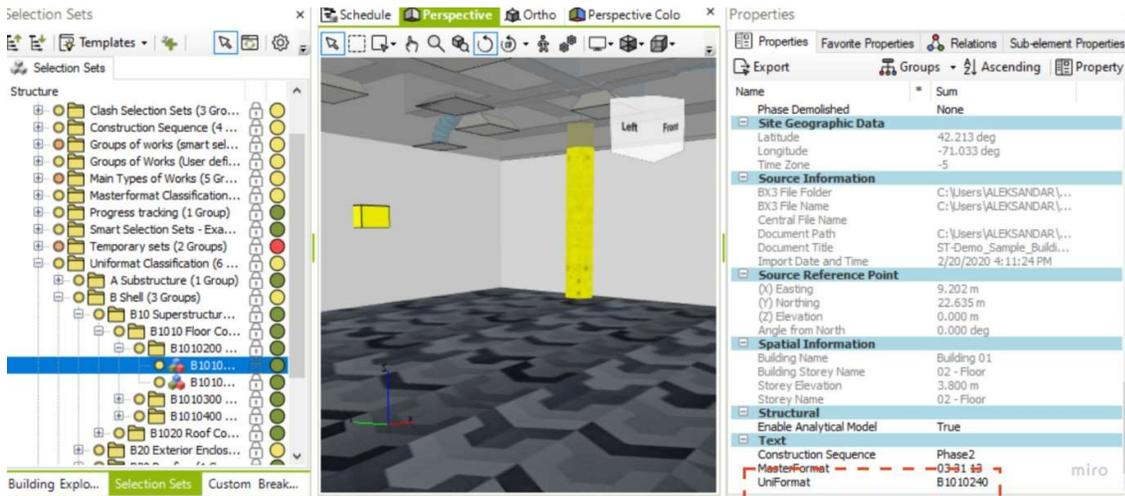
Figure 23: 3D Model element with Uniformat Classification Code and exported to Bexel Manager
