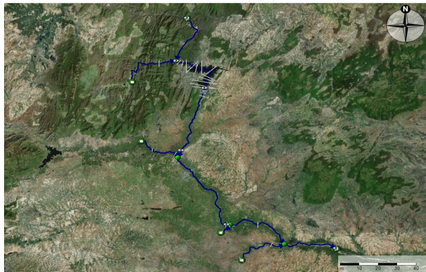
Figure 3-30: Outline of the KRS reservoir model with branches
