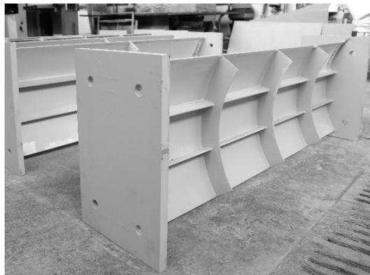
**Fig. 6.** Specimen 1C-1 with end plates welded to curved edges.
