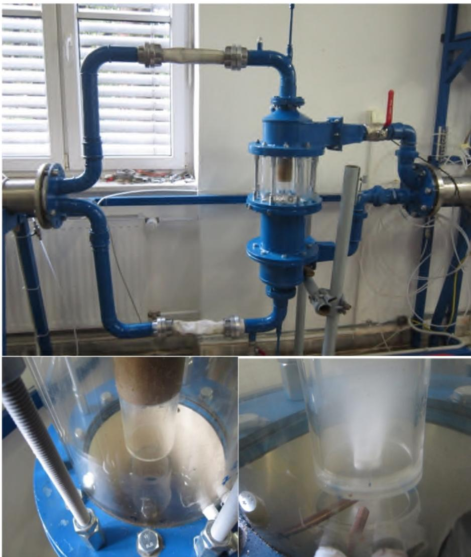
Figure 16a: Image of the pilot system III where a) is body of the pilot system III situated on the laboratory's installation, b) the inner part of the pilot system III without the nozzles at the end of the vortex finders, c) the inner part of the pilot system III during the operation.
