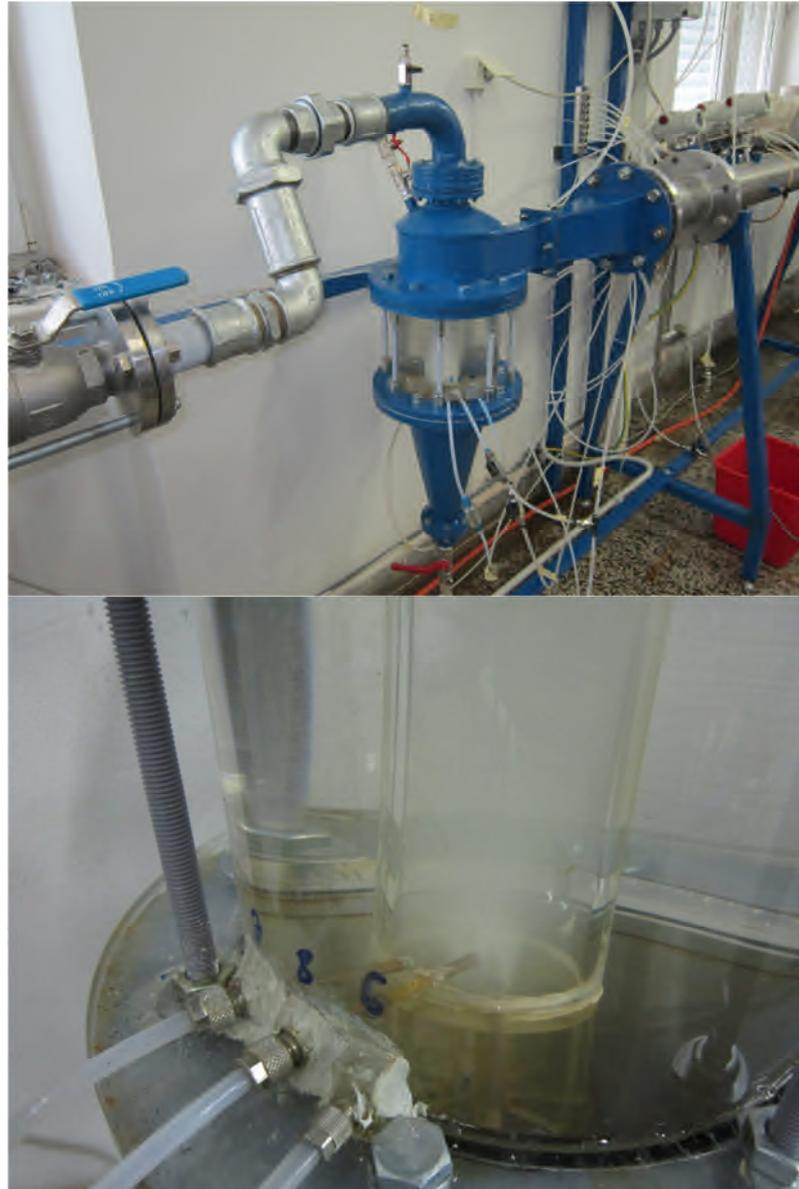
Figure 13a: Image of the pilot system II where a) is the body of the pilot system II situated on the testing area and b) cylindrical part of the pilot system II during the operation.
